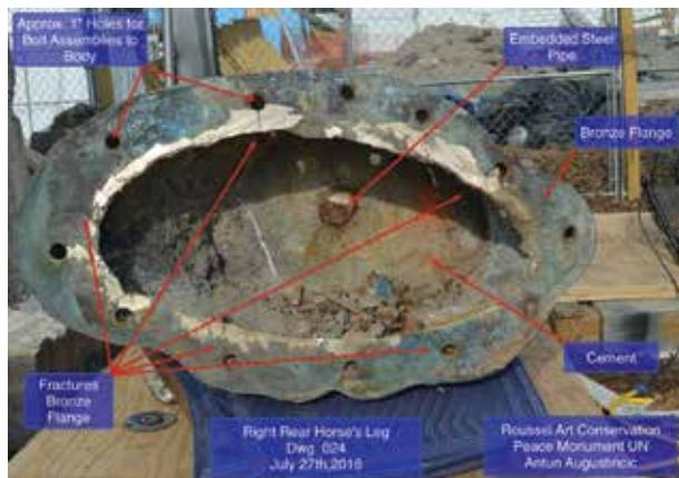
Field Diagram Right Rear Leg After Removal
